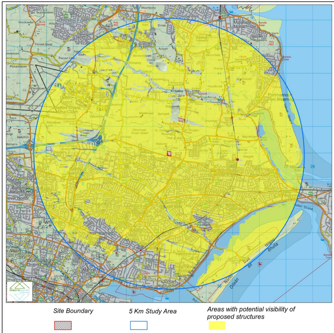
Figure 1.7 Standard (bare-ground) ZTV map (Refer to Appendix A for larger scale version)
